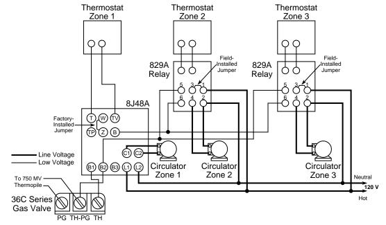
Figure 9. 8J48A - Millivolt Systems Zoned with Circulators
